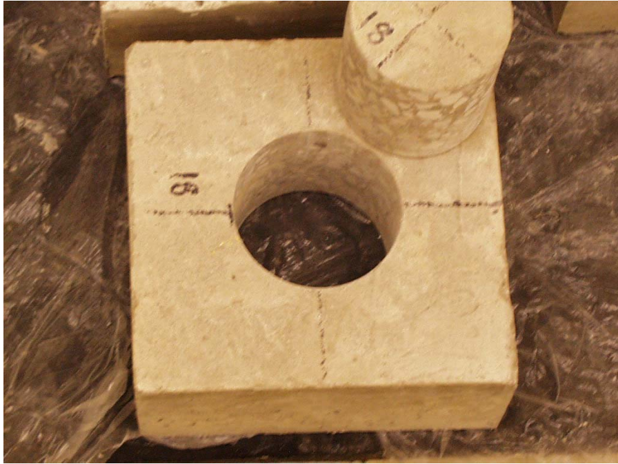
Photo 3. Close-up of cored specimen
