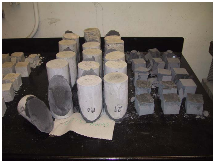
Photo 8. Slant shear bond specimens and cube specimens after testing
