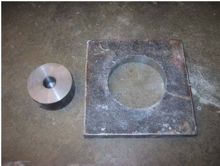
Photo 6. Top platen (left) and bottom support plate (right)
