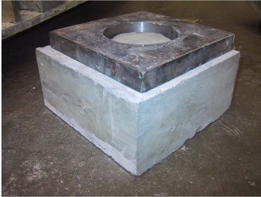
Photo 5. Support plate for punch out test shown on top of specimen
