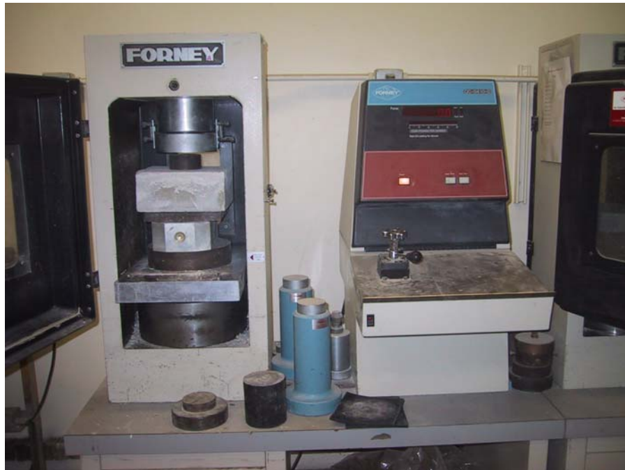
Photo 7. Compression test machine
