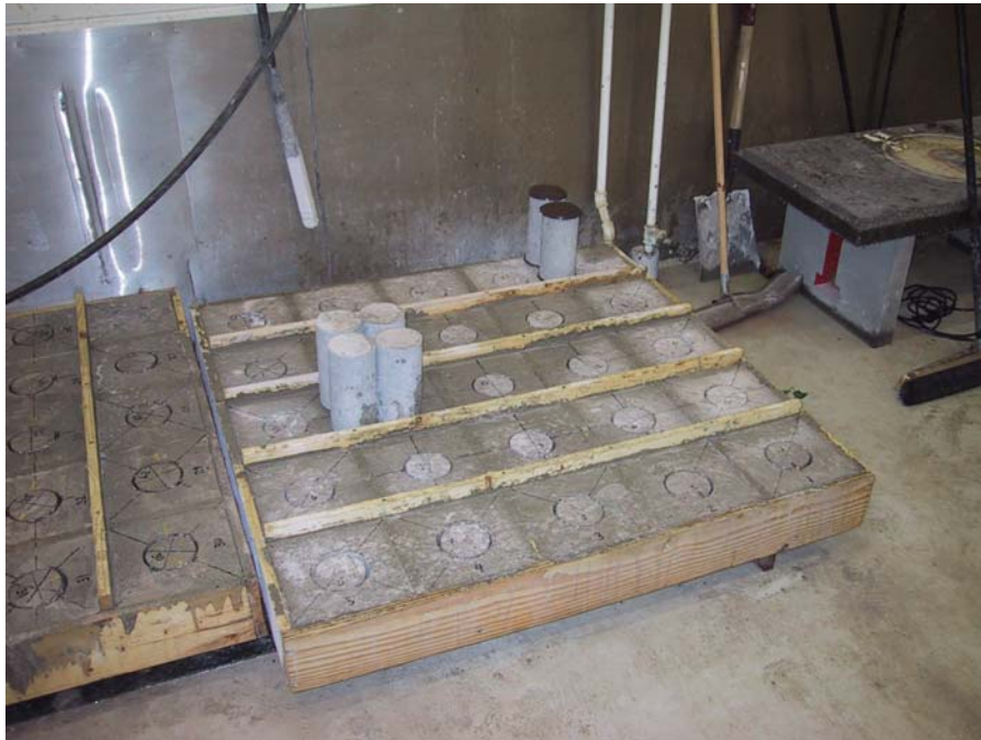
Photo 2. Cast and cored test specimens
