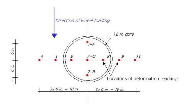
Figure 46. Locations of settlement measurements around the core
