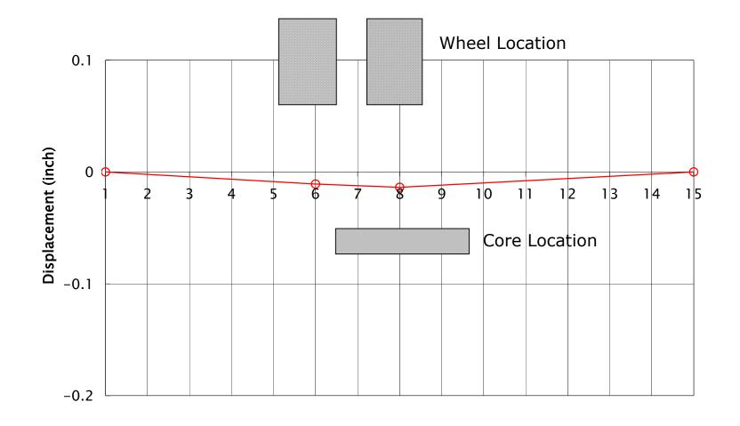
Figure 53. Displacement of core #6 section after 300 wheel passes
