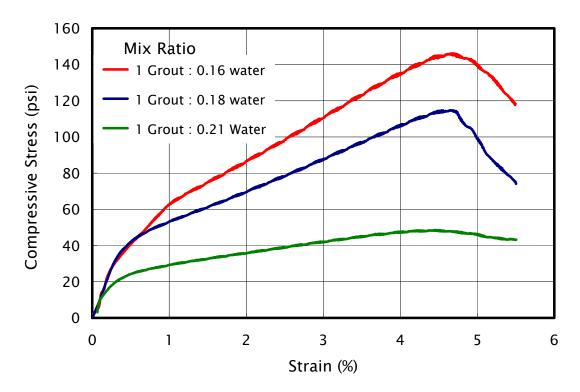
Figure 24. Compression strength of the grout at various water contents
