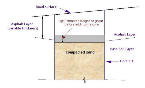
Figure 34. Use of Table 6 to estimate the height of grout (Hg)
