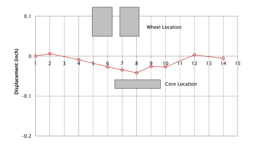
Figure 54. Displacement of core #7 section after 300 wheel passes
