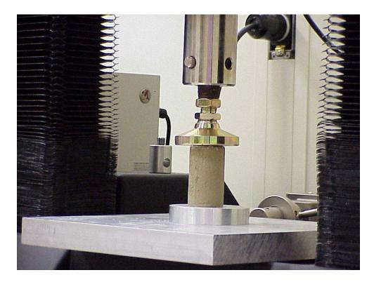
Figure 8. View of the cylindrical grout sample in a compression test
