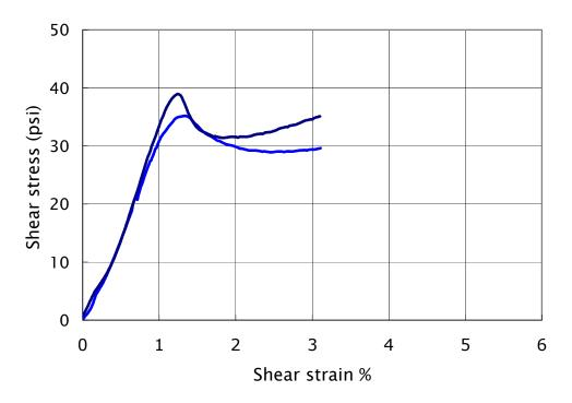
Figure 22. One-hour shear strength of the grout with 'Fast' additive
