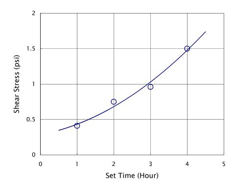
Figure 11. Increase of shear stress with time for the Duratop grout
