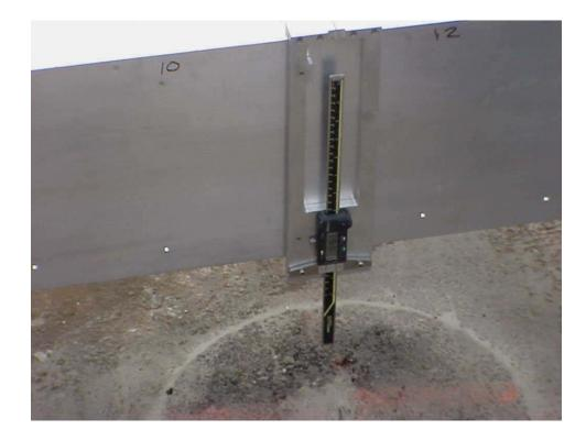
Figure 47. View of depth measurement using the depth gauge The settlement measurements along the cross sections of the cores and adjacent pavement are shown in Figures 48 to 54 for cores #1 to #7, respectively. Testing parameters and settlements measurements of these tests are also shown in Appendix A.
