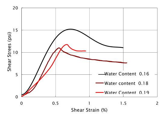
Figure 18. Results of shear tests on grouts mixed at various water contents (no additives)
