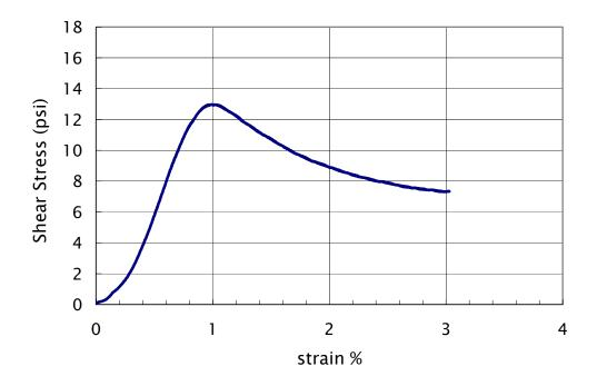
Figure 27. Result of shear test on the CeraCrete grout
