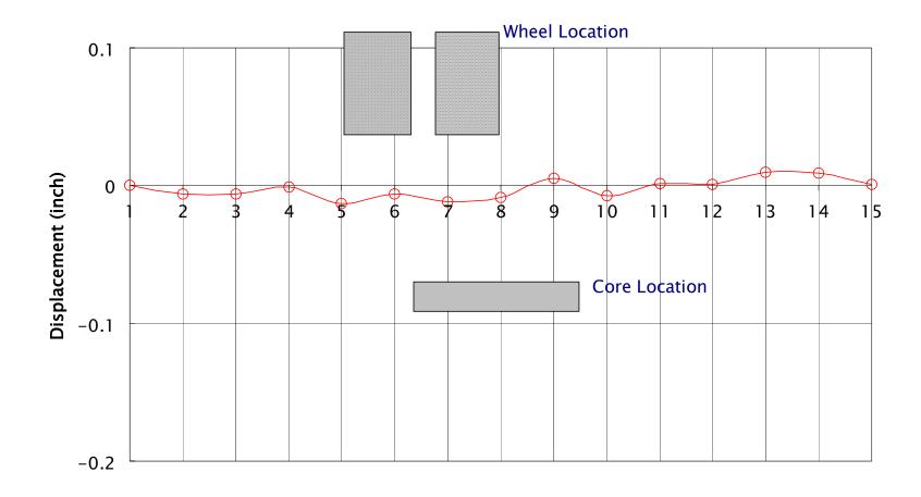
Figure 51. Displacement of core #4 section after 300 wheel passes
