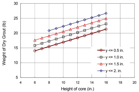
Figure 32. Weight of dry grout for 10-inch diameter cores
