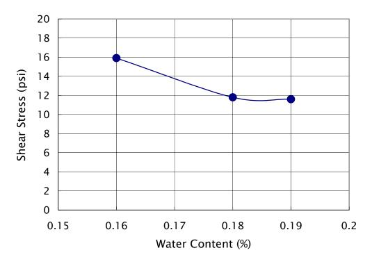
Figure 19. Effect of water content on the shear strength of grout
