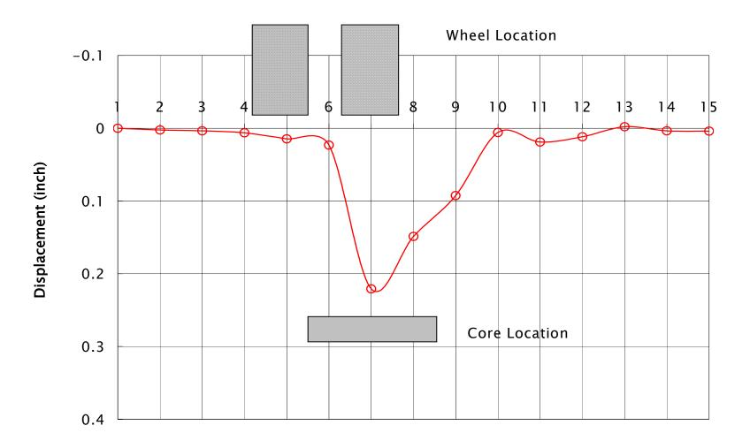
Figure 48. Displacement of core #1 section after 300 wheel passes
