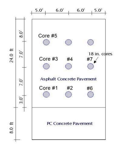
Figure 35. Layout of the field test section and locations of cores
