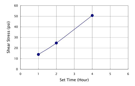
Figure 17. Increase of shear stress with setting times (water ratio 0.18, no additives)
