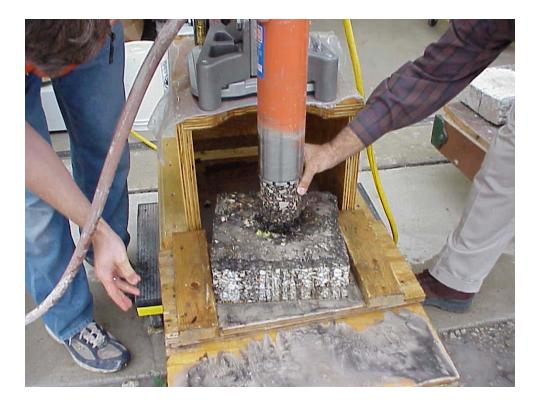
Figure 3. Retrieving the core sample from the drilling machine The grouts were mixed with various water content ratios and were tested after a setting time of one hour. Various samples were tested at longer setting periods to evaluate the strength gain of the grout with time. Figure 4 shows grout samples mixed at various water content ratios.
