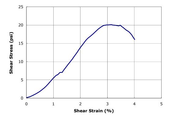
Figure 28. Shear test result on the Enbridge grout (one-hour setting time)
