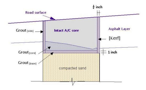
Figure 30. Typical geometry of the grout-core system
