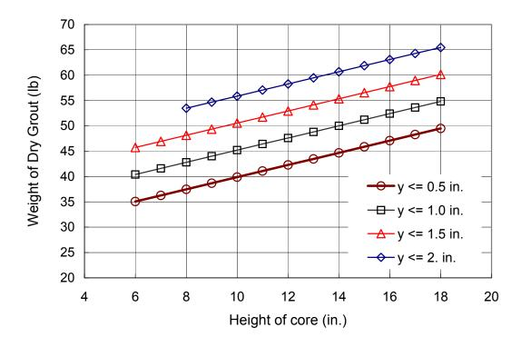
Figure 33. Weight of dry grout for 18-inch diameter cores
