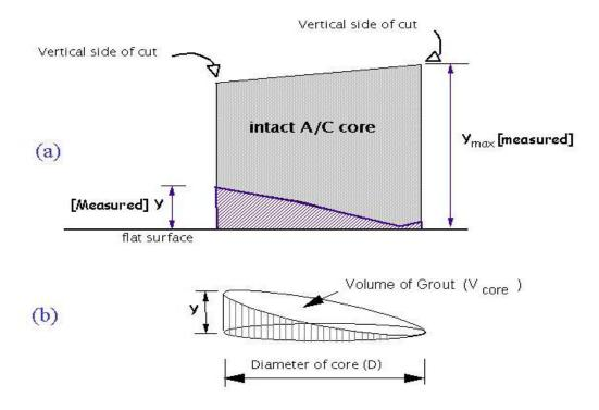
Figure 31. Estimation of quantity of grout needed for irregular base (V core)
