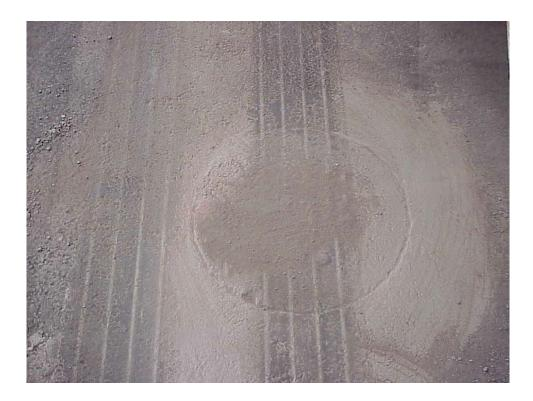
Figure 44. Location of the applied wheel load on the core
