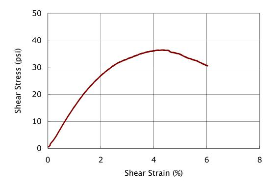
Figure 23. Shear strength after ½ hour setting time (water content 0.18, no additives)
