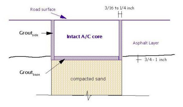
Figure 29. Ideal configuration of the grouted core
