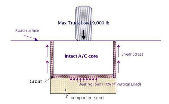
Figure 1. The grout is assumed to transfer up to 90% of the wheel load in thick cores
