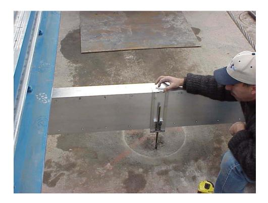
Figure 45. Measurement of core settlement using the depth profiler
