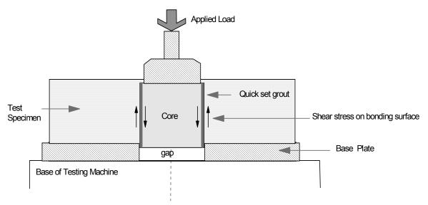
Figure 5. Schematic diagram of the shear test
