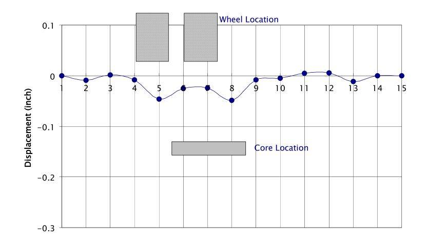
Figure 49. Displacement of core #2 section after 300 wheel passes
