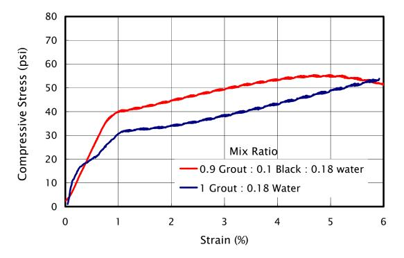
Figure 25. Compression strength of the grout with and without the "Black" additive
