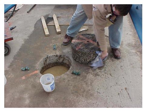
Figure 39. Cleaning the surface of the cores.
