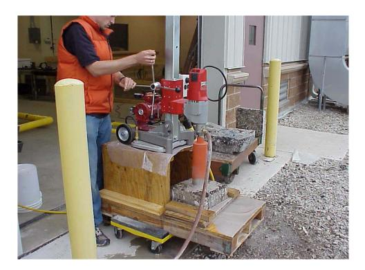
Figure 2. Drilling of the 4-inch core samples from the aged asphalt specimens
