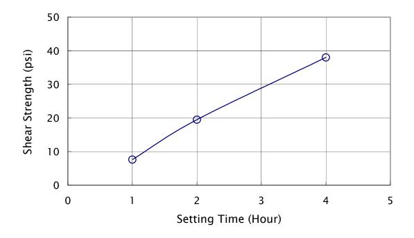
Figure 14. Increase of shear strength with time for the Rapid Set (Blue)
