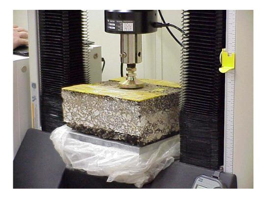
Figure 7. Application of the vertical load on the core of the asphalt sample
