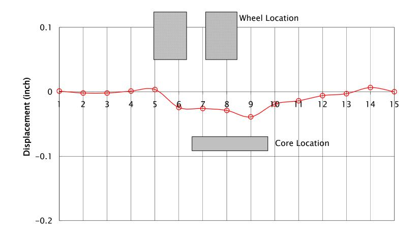
Figure 52. Displacement of core #5 section after 300 wheel passes
