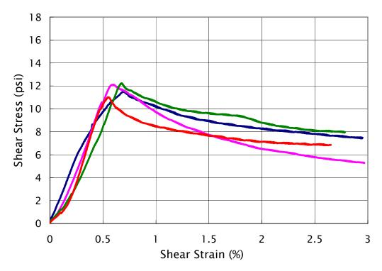
Figure 16. Shear stress results at 1-hour set time of the grout (water ratio 0.18, no additives)
